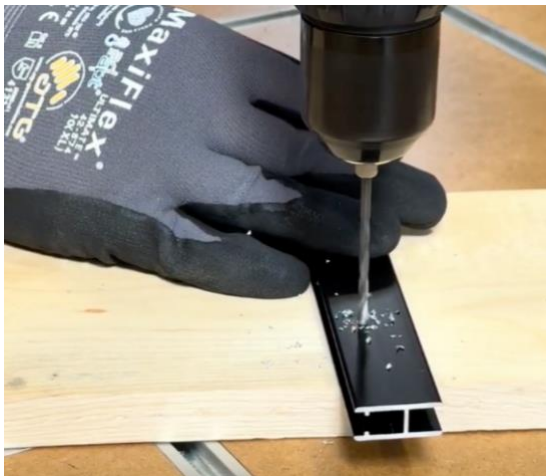
Figure 7 — Drilling the lock hole
