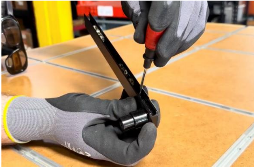
Figure 15 — Installing the push lock
